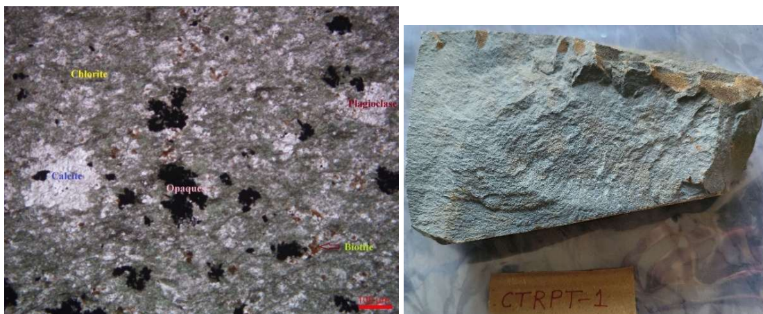
Pmg – 7.4: Photomicrograph showing association of chlorite, opaques, calcite and plagioclase and biotite as minor constituent minerals in altered basalt as seen under plane polarized light. Specimen No.: CTRPT-01, Magnification: 100X
